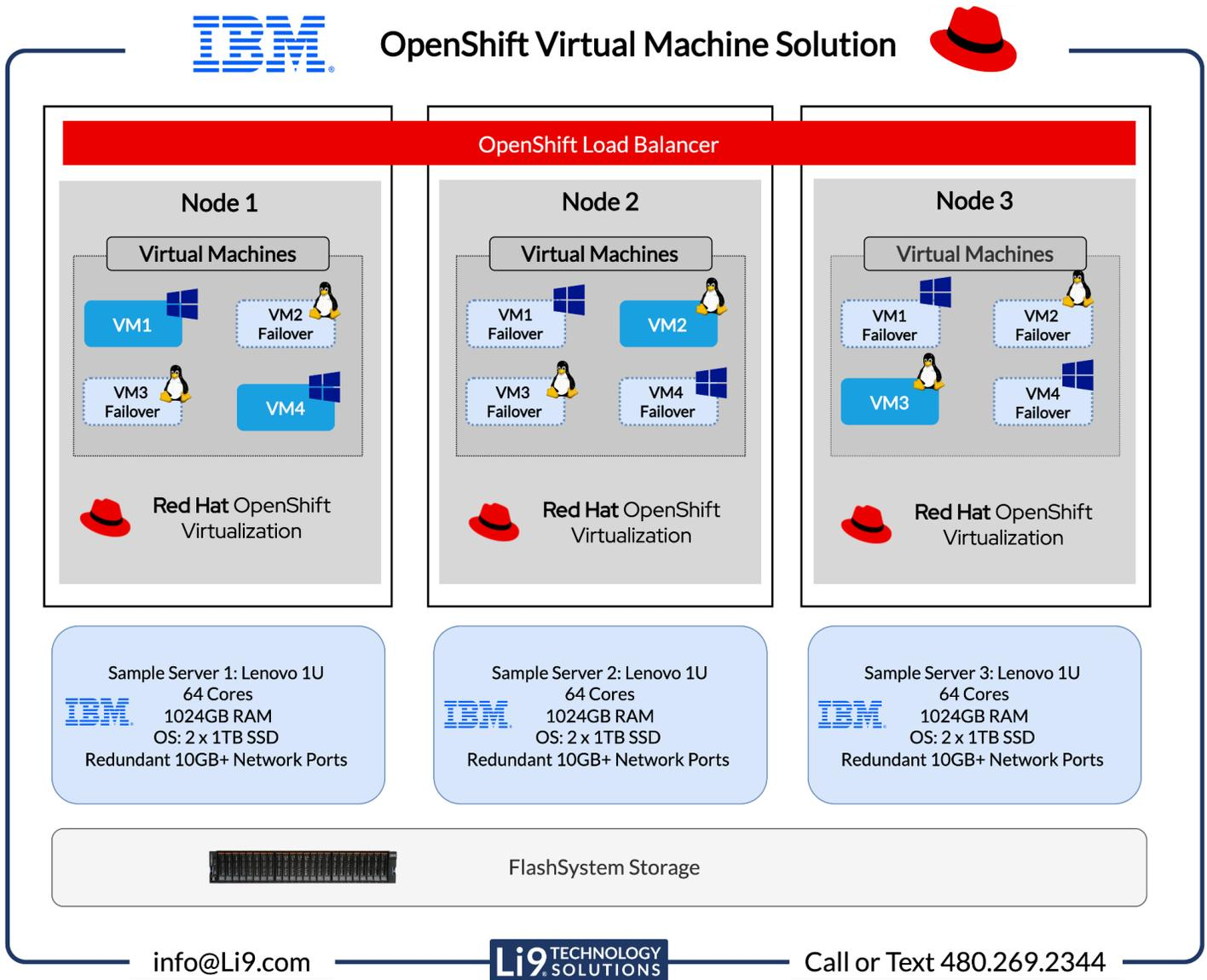
This solution delivers a 3-server (node) configuration using external data protection services with the RAID protection being handled by the IBM FlashSystem Storage.
